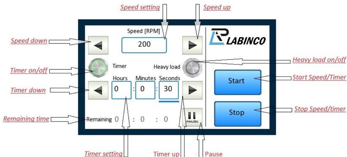
Operating instructions: Carefully unpack the unit and take off all packing materials. Choose a flat table or other suitable area for placing the Rolling bench. Check the model and catalog number indication at the rear. Check the line voltage in the room with the specified voltage on the label, this is standard 230 volts 50/60 HZ. Plug the line-plug into a suitable wall contact, with earth. Switch on the main switch. Pilot-lamp will light green if the bench is switched on.
